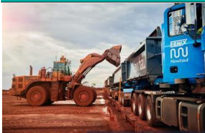
Figure 25 – Loading a 200t quad road train at Iron Ridge
